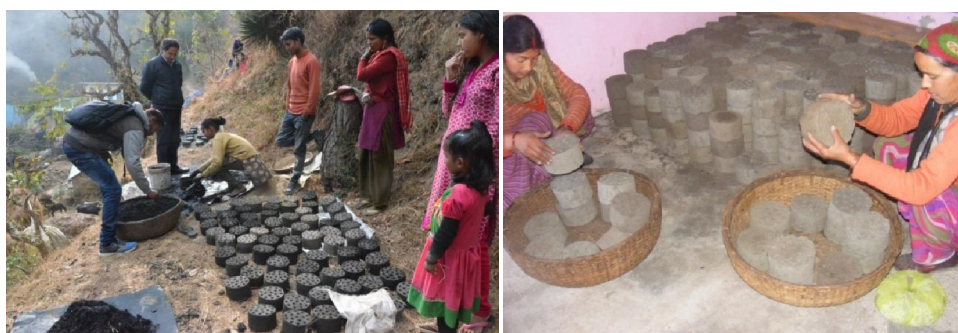
Bio-briquette preparation from dry chir-pine needles
